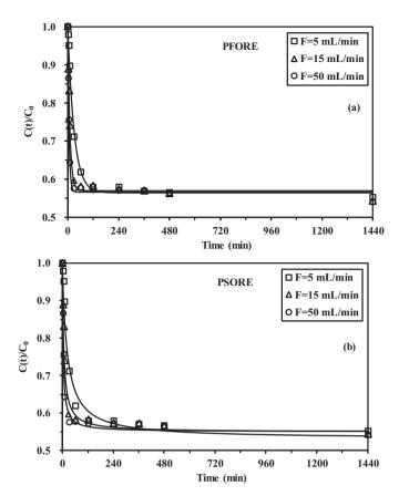
**Fig. 3.** Se(VI) uptake kinetics – Effect of flow rate ( $C_0$ : 50 mg Se L $^{-1}$ ; SD: 0.4 g L $^{-1}$ ; pH $_0$ : 2; T: 20  $\pm$  1 °C; solid line: fit of kinetic profile with the PFORE (a) and the PSORE(b)).
