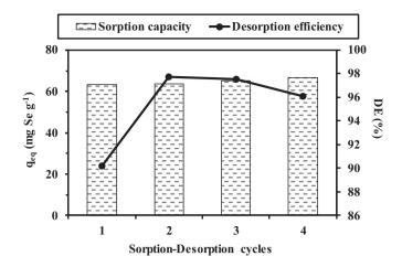
**Fig. 6.** Se(VI) desorption and sorbent recycling - Se(VI) sorption capacity and desorption efficiency (Sorption step -  $C_0$ : 100 mg Se  $L^{-1}$ ; SD: 0.8 g  $L^{-1}$ ; pH: 2; flow rate: 15 mL min $^{-1}$ ; temperature: 20  $\pm$  1 °C. Desorption step - desorption agent: 0.01 M NaOH; V: 50 mL; time: 30 min; flow rate: 15 mL min $^{-1}$ ; temperature: 20  $\pm$  1 °C).
