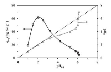
**Fig. 2.** Effect of pH on Se(VI) sorption using membrane ( $C_0$ : 100 mg Se L $^{-1}$ ; Sorbent dosage: 0.8 g L $^{-1}$ ; contact time: 24 h; flow rate: 15 mL min $^{-1}$ ; temperature, T: 20  $\pm$  1 °CC; dashed line represents pH variation during sorption).
