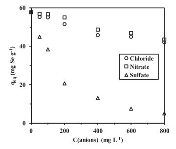
**Fig. 5.** Effect of coexisting anions on Se(VI) sorption by membranes ( $C_0$ : 100 mg L<sup>-1</sup>; SD: 1 g L<sup>-1</sup>; contact time: 24 h; pH: 2; flow rate: 15 mL min<sup>-1</sup>; temperature: 20  $\pm$  1 °C).
