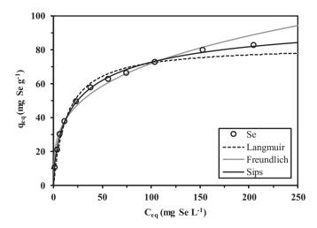
**Fig. 4.** Se(VI) sorption isotherms using membranes (SD: 0.8 g L $^{-1}$ ; contact time: 24 h; pH: 2; flow rate: 15 mL min $^{-1}$ ; T:  $20 \pm 1$  °C).
