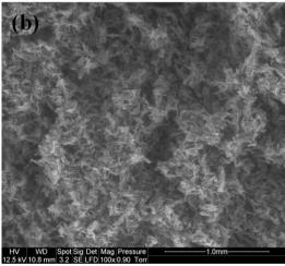
Fig. 1. Porous structure of membranes (SEM micrographs) (a) Surface and (b) Cross-section (bar: 1 mm).
