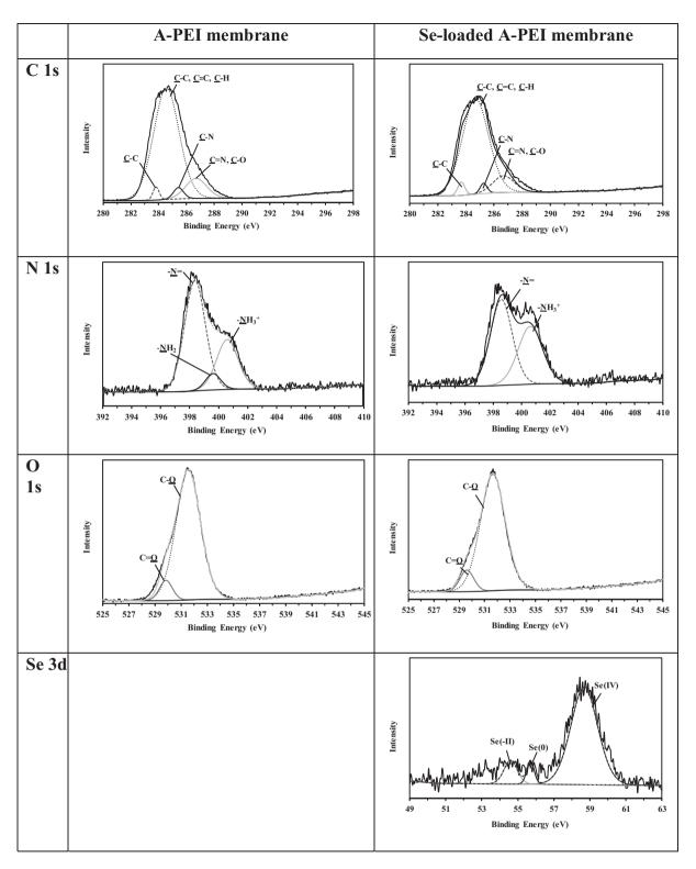
Fig. 7. High resolution C 1 s, O 1 s, N 1 s, and Se 3d core level XPS spectrum of A-PEI membrane and Se(VI)-loaded A-PEI membrane.
