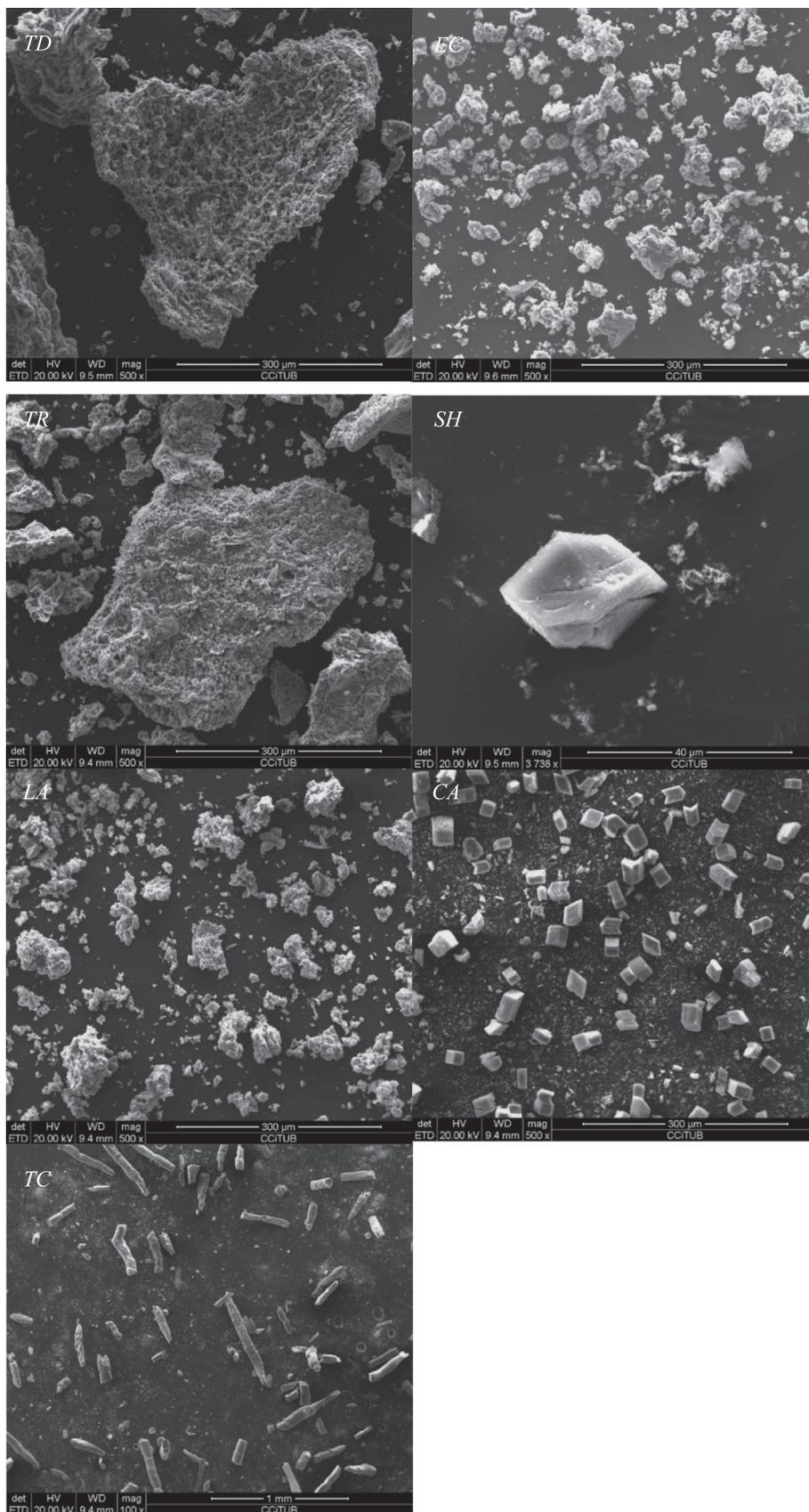
Fig. 2. SEM images from the calcined residues.
