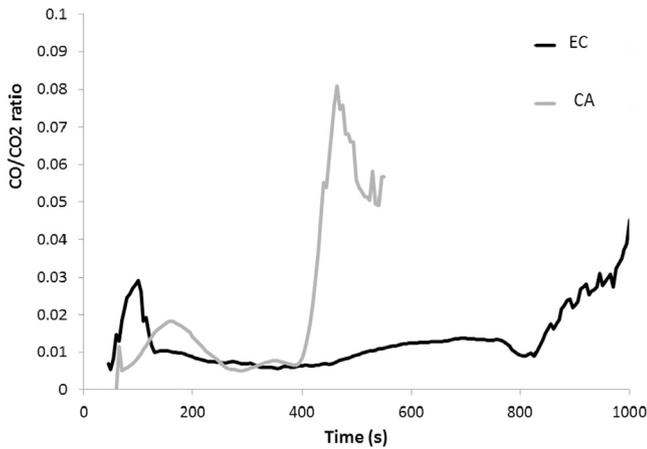
Fig. 11. CO/CO<sub>2</sub> ratio versus time for two wood samples in cone calorimeter tests.
