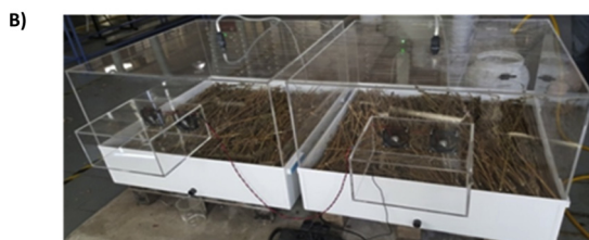
Fig. 2. A) Field retting (left: non-retted stems; middle: 3 weeks retted stems; right: 9 weeks retted stems). B) Lab-scale pilot units used for a controlled and accelerated retting.
