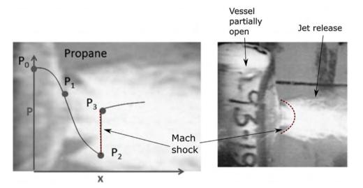
Fig. 2. Pressure Distribution along axis of fish mouth opening on vessel with image of jet showing Mach shock standing beyond opening (vessel D =0.61 m, propane, failure pressure approximately 20 Barg) (Laboureur et al., 2015).
