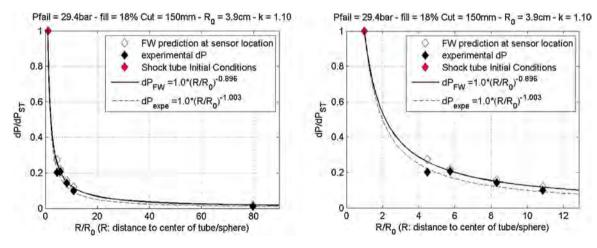
Fig. 13. Measured Peak Overpressure vs scaled distance R/Ro where Ro = radius of sphere based on vapour space volume along the tube weakened length (left: full scale along R/Ro; right: zoom on the first 4 sensors).
