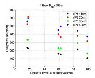
**Fig. 15.** Maximum overpressure measured above the vessel at 4 different distances, against liquid fill level, for cases of similar failure pressure (17 bar  $< P_{fail} < 19$  bar) and cut length (150 mm).
