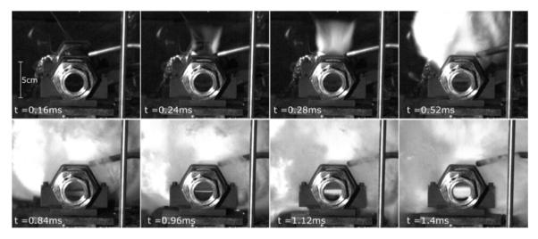
**Fig. 11.** Axial end view with direct high speed imaging (Camera Phantom V711,  $P_f = 28bar$ ; fill = 56%;  $L_c = 75mm$ ).
