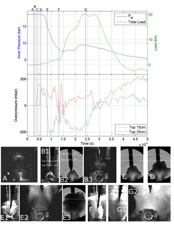
**Fig. 14.** Chronology of a BLEVE through physical measurements and high speed imaging ( $P_{fail} = 18.6bar$ ,  $\Phi_{liq} = 56\%$ ,  $L_w = 75mm$ ).
