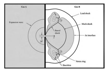
Fig. 1. the starting of a lead shock from the transient flow from an opening in a pressurized container (from Radulescu and Law, 2007).
