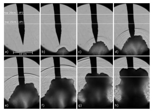
**Fig. 12.** Radial view with shadowgraph high speed imaging (Camera Phantom V2512,  $\Delta t = 120 \mu s$ ,  $P_{fail} = 19.3$  bar,  $\Phi_{lia} = 84\%$ ,  $L_w = 150$  mm).
