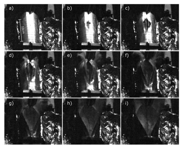
**Fig. 10.** Top view with direct high speed imaging (Camera Phantom VEO710,  $\Delta t = 52\mu s$ ,  $P_f = 19.3bar$ ; fill = 84%;  $L_c = 150mm$ ).
