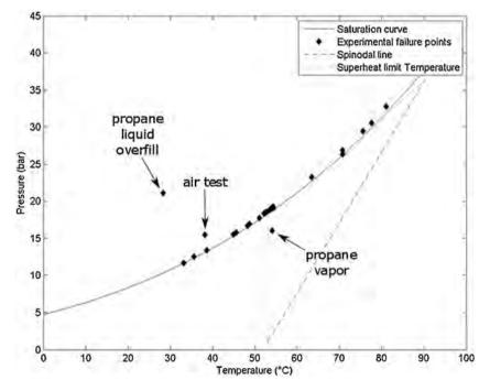
Fig. 8. Failure Temperatures and Pressures compared to saturation pressure curve for propane.
