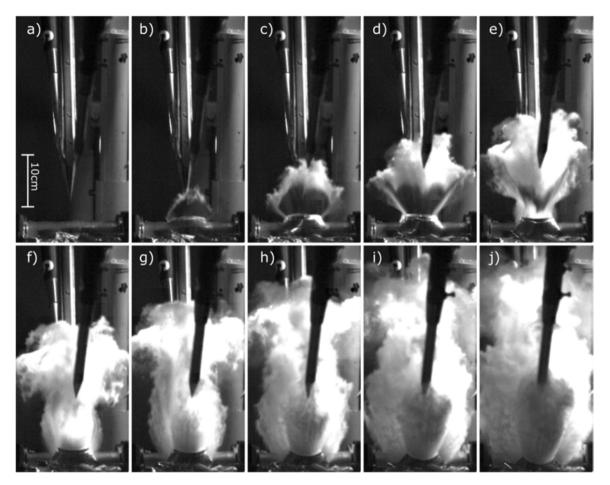
**Fig. 9.** Side view with direct high speed imaging (camera Photron SA3,  $\Delta t = 200 \mu s$ ,  $P_f = 18.6 bar$ ; fill = 56%;  $L_c = 75 mm$ ).
