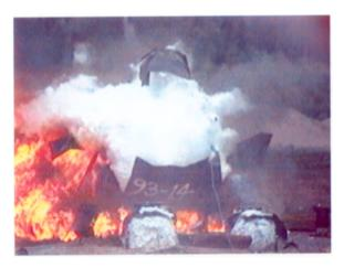
**Fig. 5.** 0.4 m<sup>3</sup> pressure vessel suffering a BLEVE. Failure runs along top of vessel and turns circumferentially at the ends. This vessel eventually flattened on the ground.
