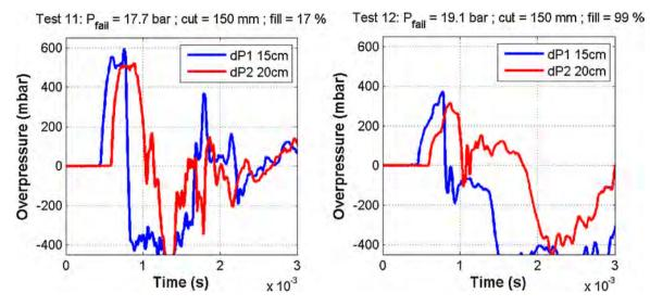
Fig. 16. Pressure signals from two sensors above the vessel (15 and 20 cm) for two cases of similar failure pressure and cut length, but different liquid fill level.
