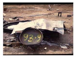
Fig. 6. 0.4 m<sup>3</sup> pressure vessel after suffering a BLEVE. Failure runs.
