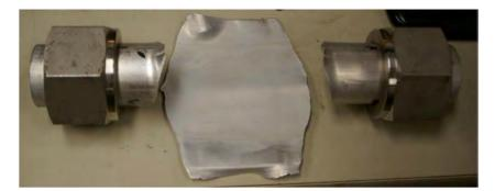
Fig. 4. image of failed tube with separated part of wall flattened on blast plate. Weakened length is the upper and lower free edges of the flattened part.
