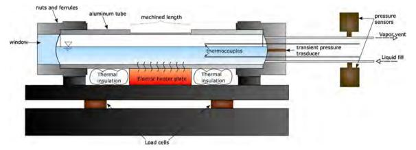
Fig. 7. Schematic diagram of tube apparatus (tube D =50 mm).
