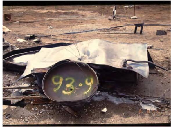
Fig. 6. 0.4 m<sup>3</sup> pressure vessel after suffering a BLEVE. Failure runs.
