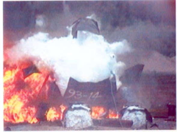
Fig. 5. 0.4 m<sup>3</sup> pressure vessel suffering a BLEVE. Failure runs along top of vessel and turns circumferentially at the ends. This vessel eventually flattened on the ground.
