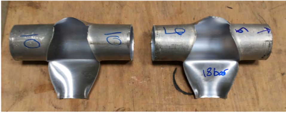
Fig. 7. Two samples of tubes that failed while filled with both liquid and vapour propane.
