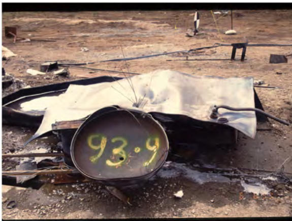
Fig. 4. 0.4 m 3 pressure vessel after suffering a BLEVE. Failure runs along top of vessel and turns circumferentially at the ends. Cylinder flattened on the ground.
