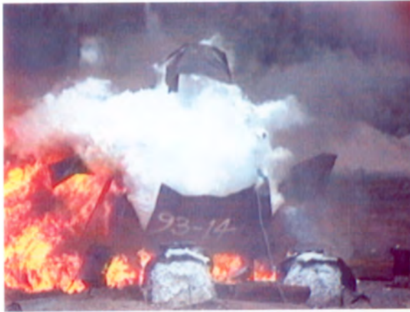
Fig. 3. 0.4 m 3 pressure vessel suffering a BLEVE. Failure runs along top of vessel and turns circumferentially at the ends. This vessel eventually flattened on the ground.
