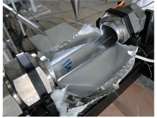
Fig. 1. Image of opened tube with flattened part still attached to ends. Failure runs along top of tube and then turns circumferentially at the ends of the weakened length.
