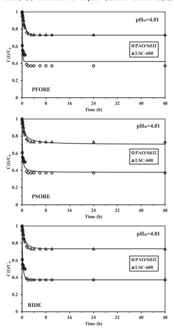
**Fig. 6.** Comparison of kinetic profiles for Ga(III) sorption using PAO/SiO $_2$  sorbent and LSC-600 commercial resin (C $_0$ : 25 mg Ga L $^{-1}$  – 0.364 mmol Ga L $^{-1}$ ; SD: 0.25 g L $^{-1}$ ; pH $_0$ : 4.12; T: 25 °C; Ga $_2$ O $_3$  dissolved in NaOH solution).
