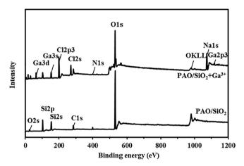
Fig. 4. XPS spectra of PAO/SiO<sub>2</sub> before and after Ga(III) loading (full survey).
