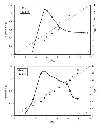
**Fig. 5.** Effect of pH on sorption capacity for Ga(III) using  $PAN/SiO_2$  and pH variation during metal sorption: (a)  $Ga_2O_3$  solution, (b)  $Ga(NO_3)_3$  solution (Sorbent dosage, SD:  $280\,\mathrm{mg}~\mathrm{L}^{-1}$ ;  $C_0$ :  $0.567\,\mathrm{mmol}\,\mathrm{Ga}~\mathrm{L}^{-1}$ ; T:  $25\,^{\circ}\mathrm{C}$ ; agitation speed:  $150\,\mathrm{rpm}$ ; contact time:  $48\,\mathrm{h}$ ).
