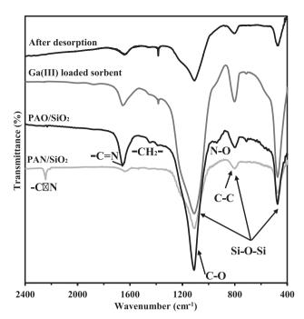
**Fig. 2.** FTIR spectra of PAN/SiO<sub>2</sub>, and PAO/SiO<sub>2</sub> for identifying the chemical modifications of the support; for amidoxime sorbent: spectra after Ga(III) sorption and after metal desorption (scaled to the wavenumber range:  $400-2400 \, \mathrm{cm}^{-1}$ ).
