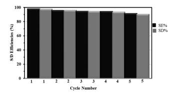
**Fig. 11.** Sorbent recycling at different volumetric ratios between the sorption step and the desorption step  $(V_{sorpt.}/V_{des.})$  (Sorption step:  $C_0$ : 50 mg Ga L<sup>-1</sup>; pH 4; SD: 1 g L<sup>-1</sup>; contact time: 24 h – Desorption step: 1.5 M HCl solution; contact time: 2 h; SD: 0.9 g L<sup>-1</sup>; T: 25 °C).
