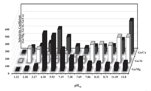
Fig. 12. Ga(III) sorption on PAO/SiO<sub>2</sub> from multi-metal solutions – Selectivity coefficients in function of equilibrium pH (SD: 0.825 g L<sup>-1</sup>; C<sub>0</sub>: 1.8 (  $\pm$  0.2) mmol L<sup>-1</sup> for Ca(II), Mg(II) and Al(III); 1.01 mmol L<sup>-1</sup> for Ga; pH<sub>0</sub>: 1.0-13.0; contact time: 6 h; T:  $22 \pm 1$  °C).
