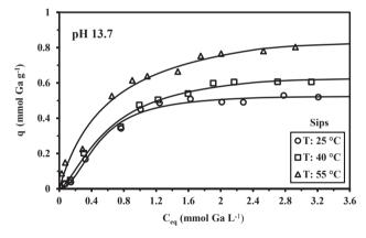
Fig. 10. Ga(III) sorption isotherms at different temperatures using PAO/SiO $_2$  sorbent at pH 13.7 – Comparison of isotherm models (solutions prepared by dissolving  $Ga_2O_3$  in NaOH solution).
