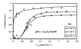
Fig. 9. Ga(III) sorption isotherms at different temperatures using PAO/SiO<sub>2</sub> sorbent at pH 4 using Ga(III) solutions prepared by dissolving of  $Ga_2O_3$  in NaOH solution or  $Ga(NO_3)_3$  salt.
