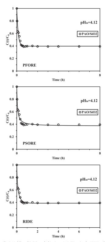
**Fig. 7.** Modeling of Ga(III) uptake kinetics on PAO/SiO $_2$  using the PFORE and RIDE equations (C $_0$ : 40 mg Ga L $^{-1}$  – 0.595 mmol Ga L $^{-1}$ ; SD: 0.25 g L $^{-1}$ ; pH $_0$ : 4.12; T: 25 °C; Ga(NO $_3$ ) $_3$  salt).
