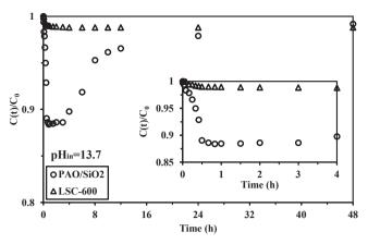
**Fig. 8.** Comparison of kinetic profiles for Ga(III) sorption using PAO/SiO<sub>2</sub> sorbent and LSC-600 commercial resin ( $C_0$ : 90 mg Ga L $^{-1}$  – 1.326 mmol Ga L $^{-1}$ ; SD: 0.3 g L $^{-1}$ ; pH<sub>0</sub>: 13.7; pH<sub>eq</sub>: 12.13; T: 25 °C).
