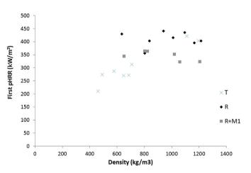
Fig. 19. First pHRR versus density for woods and wood-plastic composites (small samples  $7 \times 7 \times 1$  cm<sup>3</sup>).
