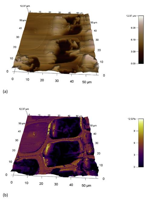
Fig. 7. AFM images of a pine sample with polyester resin: (a) topography, (b) elastic modulus.
