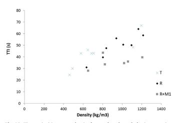
Fig. 18. Time-to-ignition versus density for woods and wood-plastic composites (small samples  $7 \times 7 \times 1 \text{ cm}^3$ ).
