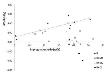
Fig. 22. Change in THR versus impregnation ratio for all wood-plastic composites.
