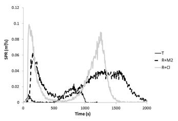
Fig. 23. Smoke production rate curves in cone calorimeter tests for pine (transverse orientation) and some pine-plastic composites.
