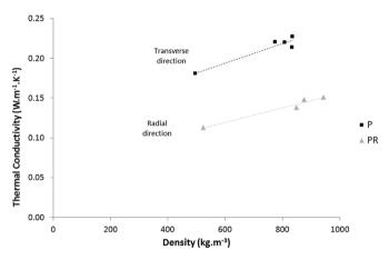
Fig. 9. Thermal conductivity versus density for woods and wood-plastic composites based on pine (radial and transverse orientation).
