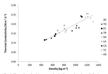
Fig. 8. Thermal conductivity versus density for woods and wood-plastic composites (small samples  $7 \times 7 \times 1$  cm<sup>3</sup>).
