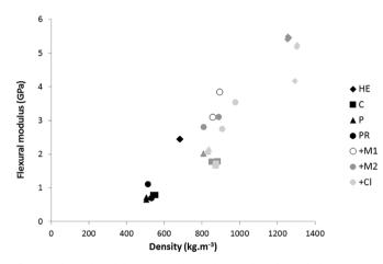
Fig. 15. Flexural modulus versus density for woods and wood-plastic composites based on pine, beech and chestnut species.
