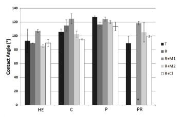
**Fig. 12.** Contact angle (°) with water for several wood samples modified or not with resins (\* PR sample impregnated with R resin was not prepared).
