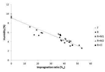
Fig. 10. Humidity versus impregnation ratio for all woods and wood-plastic composites.
