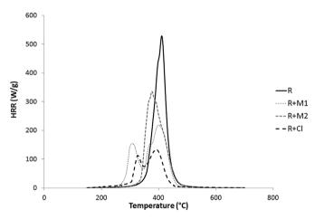
Fig. 3. Heat release rate versus temperature for studied resins from PCFC analyses.
