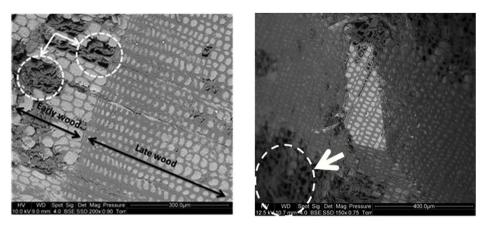
Fig. 5. SEM pictures showing pine wood impregnated by the chlorinated resin: surface (left) and at a depth of 1 cm (right) – The white arrow points out a non-impregnated zone.
