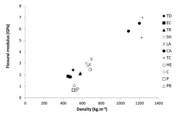
Fig. 14. Flexural modulus versus density for all studied woods.
