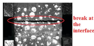
**Figure 4.** Crack growth at interface during tensile test
