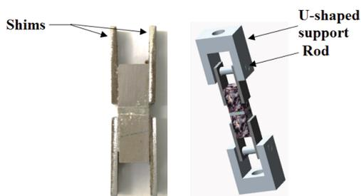
**Figure 2.** Experimental device for direct tensile test
