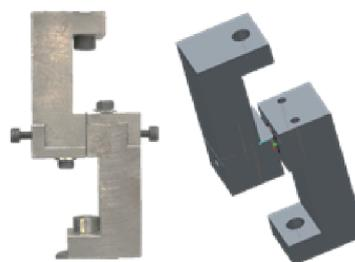
**Figure 3.** Experimental device for direct shear test
